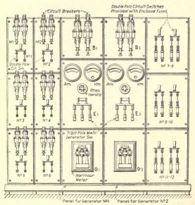
Fig. 213.—Front view of the five-panel direct-current switchboard.
